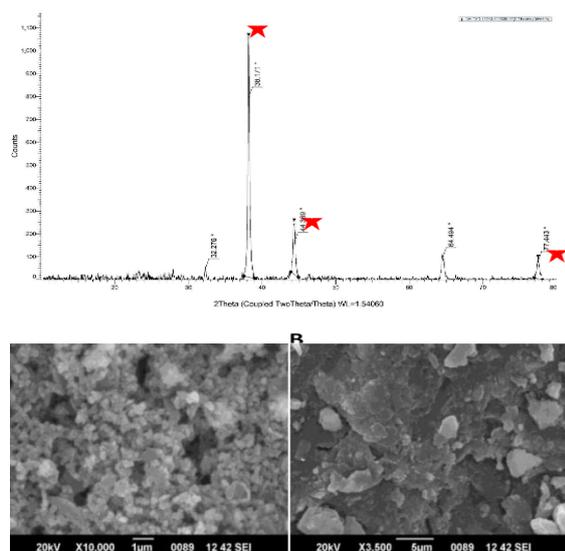
**Fig. 6.** SEM images of AgNPs(A) from aqueous extract (B) from ethanol extract
