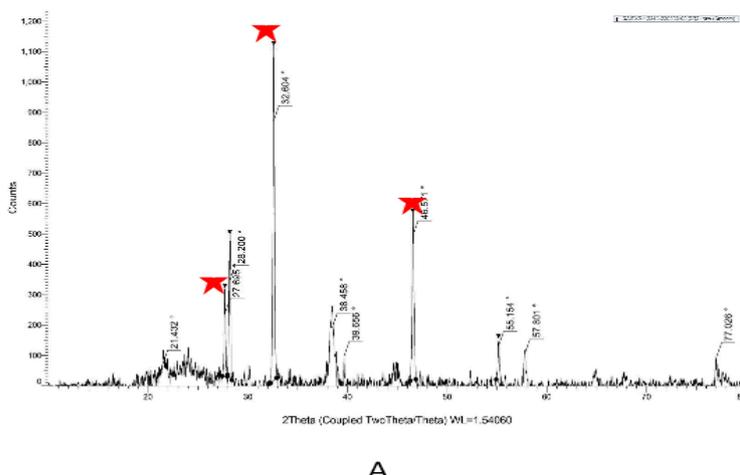
**Fig. 5.** XRD spectra of AgNPs(A) from aqueous extract (B) from ethanol extract
